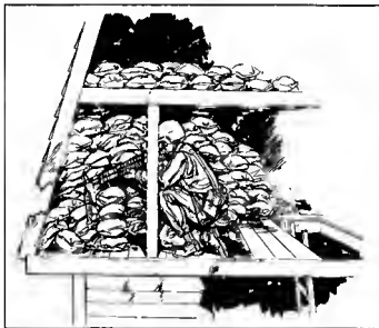
Figure 5-41. Firing platform built under roof.
